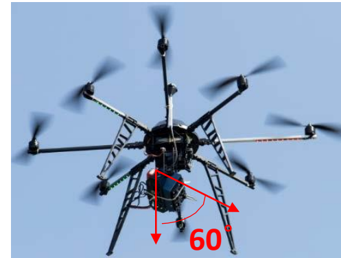
Oblique viewing from an unmanned aerial vehicle (UAV)
